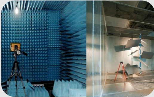
Anechoic chamber and reverberation chamber
